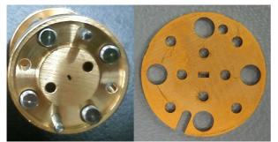
Fig. 1 Photograph of test port (WM-864) and Standard line (WM1651)
