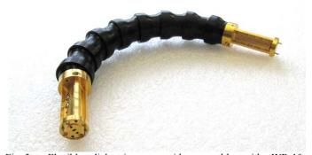
Fig. 3. Flexible dielectric waveguide assembly with WR-10 interfaces (300 mm total length, 7 standard segments).
