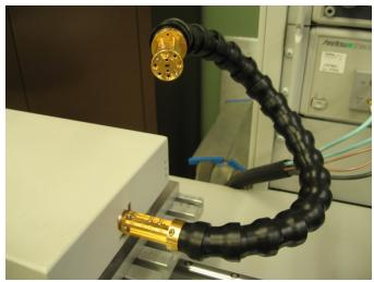
Fig. 4. Flexible dielectric waveguide assembly with WR-10 interfaces connected to a VNA frequency extender unit (575 mm total length, 18 standard segments).
