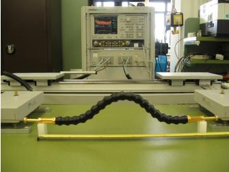
Fig. 5. 575 mm dielectric waveguide assembly with WR-10 interfaces connected between two VNA frequency extender units.
