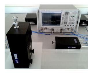
Fig. 2. The 750 GHz to 1.1 THz VNA system used for the measurements
