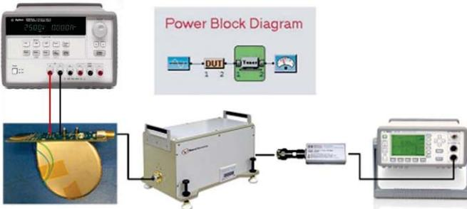
Fig. 4. Diagram of the load pull test setup. Shown are the implantable device (with interface board in place of header/antenna) serving as both signal source and DUT, a Keysight E3631A DC Power Supply, a Maury MT981A Automated Tuner, a Keysight E4419B Power Meter with Power Sensor, and the Maury Automated Tuner System Software v.5.0.
