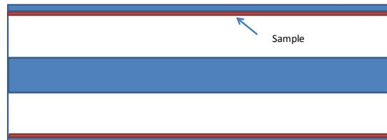
Fig. 2. The proposed installation method of the sample in the coaxial transmission line.
