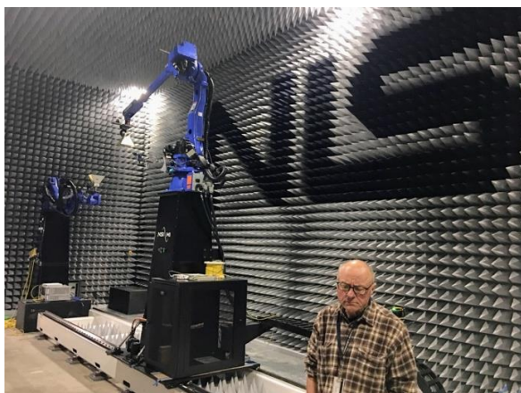
NIST hosted facilities tours for all interested ARFTG symposium attendees. Pictured above is a new robotic antenna system for very precise mm-wave measurements.
